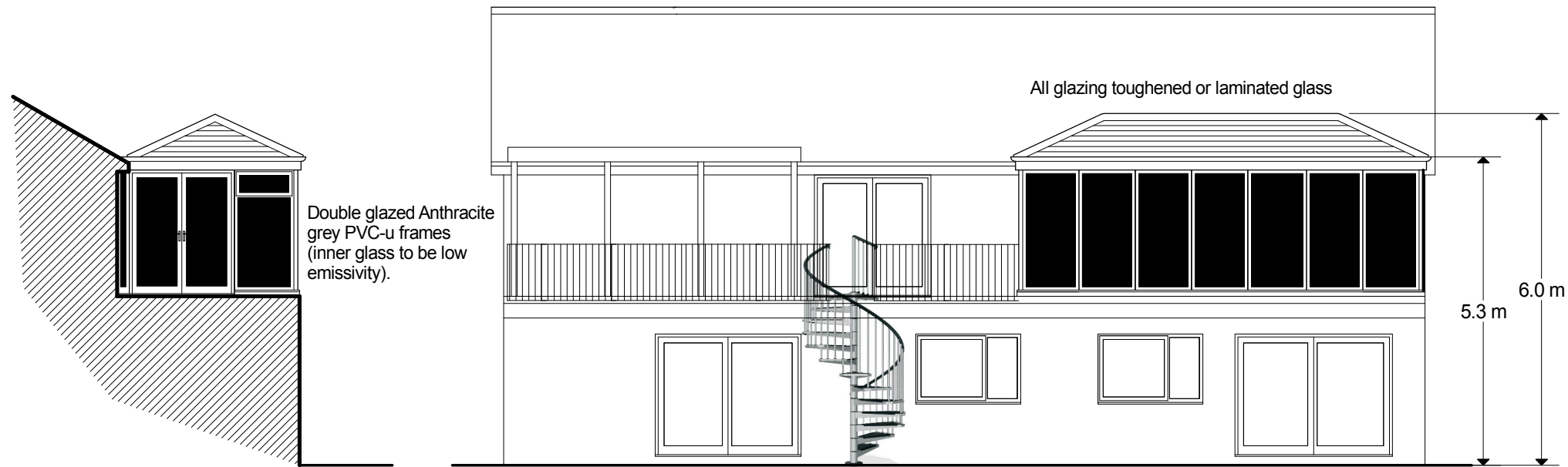
NORTH ELEVATION AS BUILT
