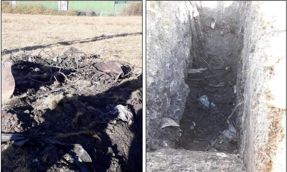
Figure 2 - Images displaying anthropogenic material in opencast mine backfill in TP17
