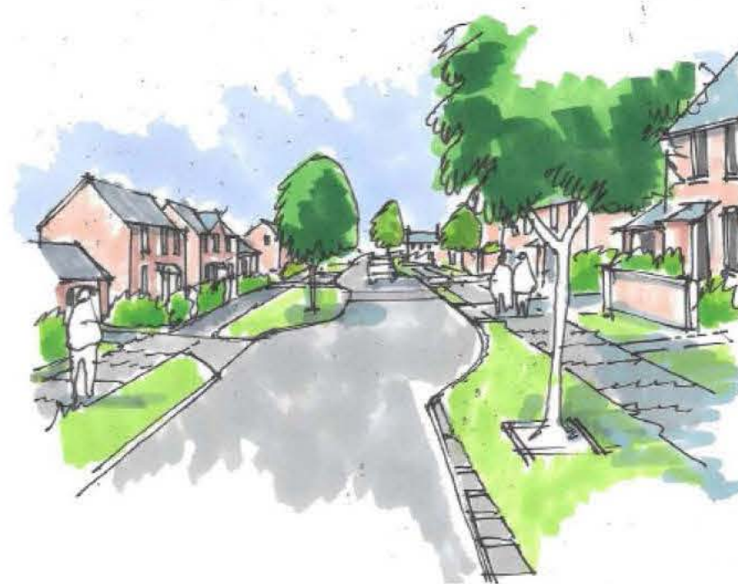
(Left) A secondary residential access road showing traffic calmed road alignment and integrated landscaping
