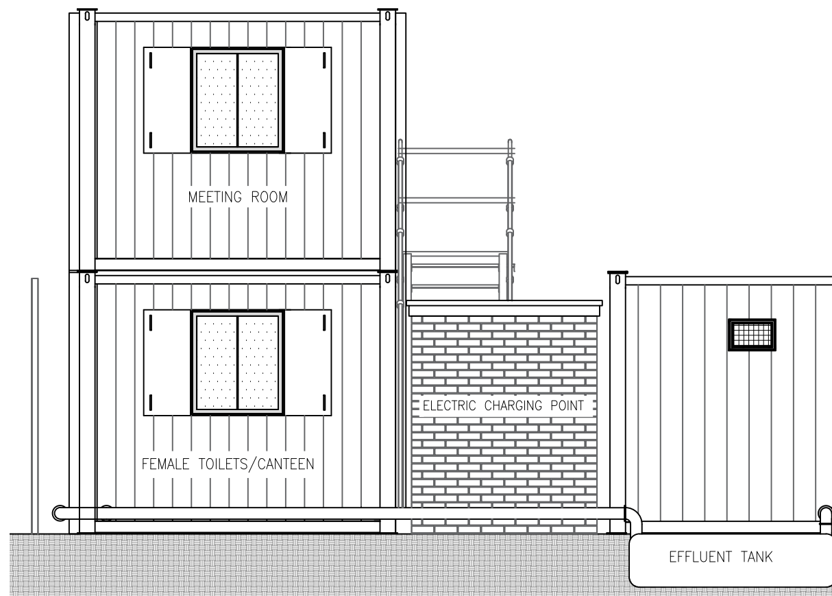
TANK PLACEMENT ELEVATION 1:50
