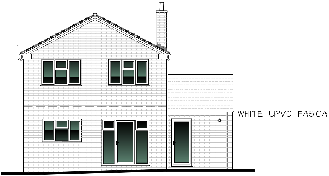
EXISTING REAR (W) ELEVATION 1:100
