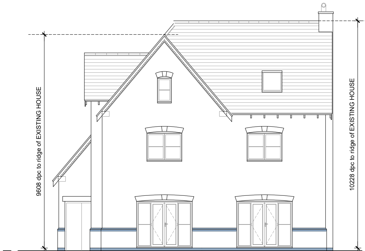
EXISTING REAR ELEVATION
