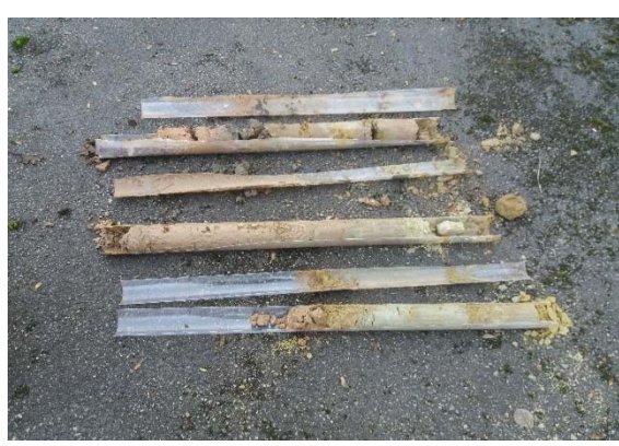
Photo 6: Image showing the material recovered from WS08
