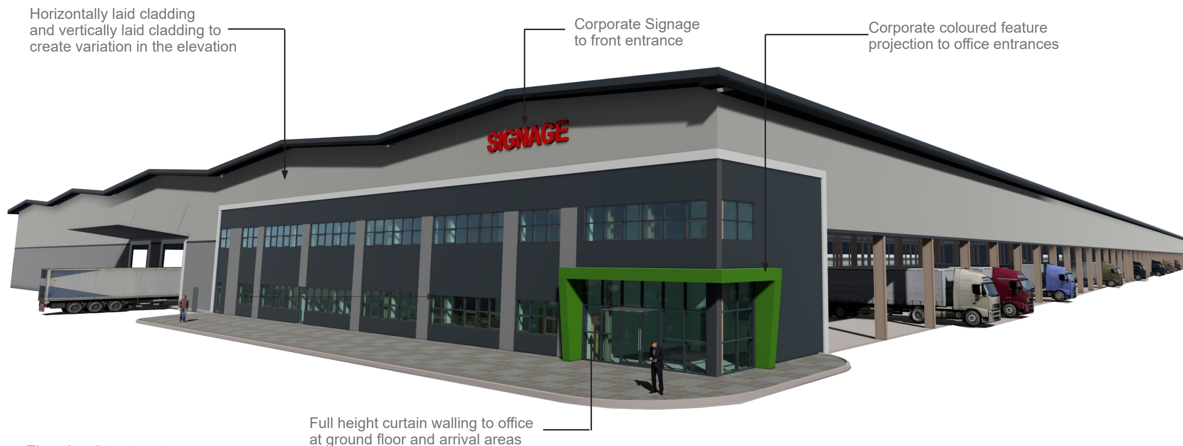
Above: Warehouse Elevational treatment
