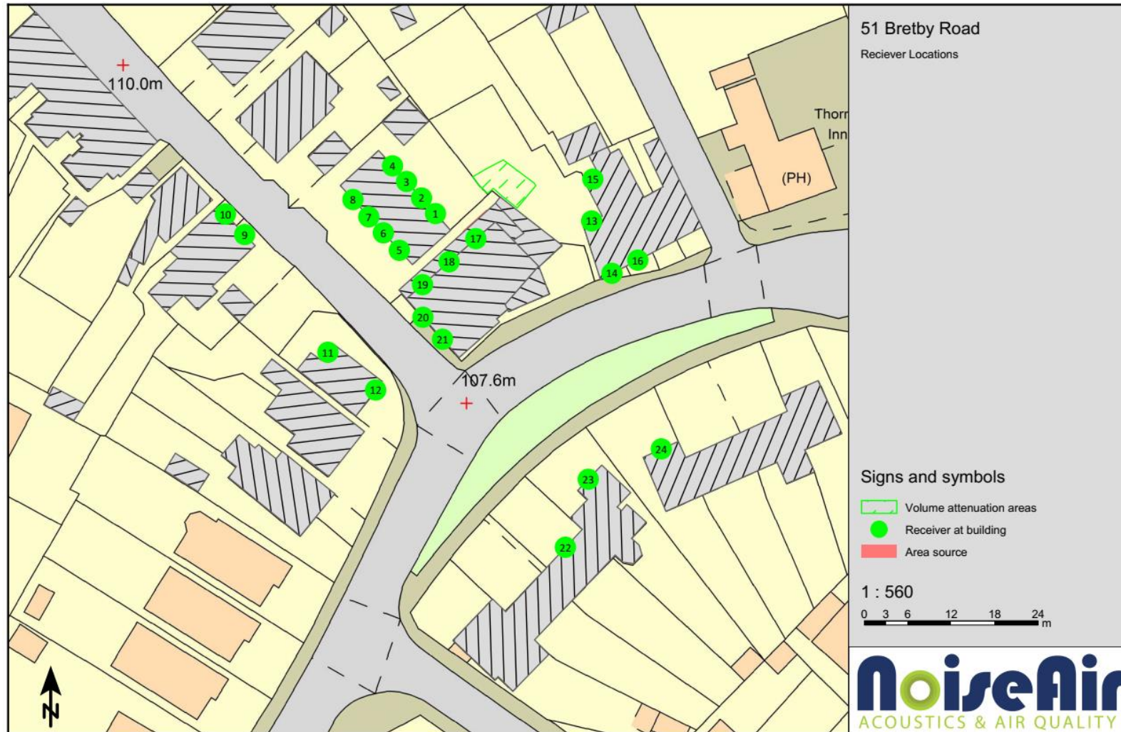
Figure 7: Illustration of the 3D sound model receptor locations.
