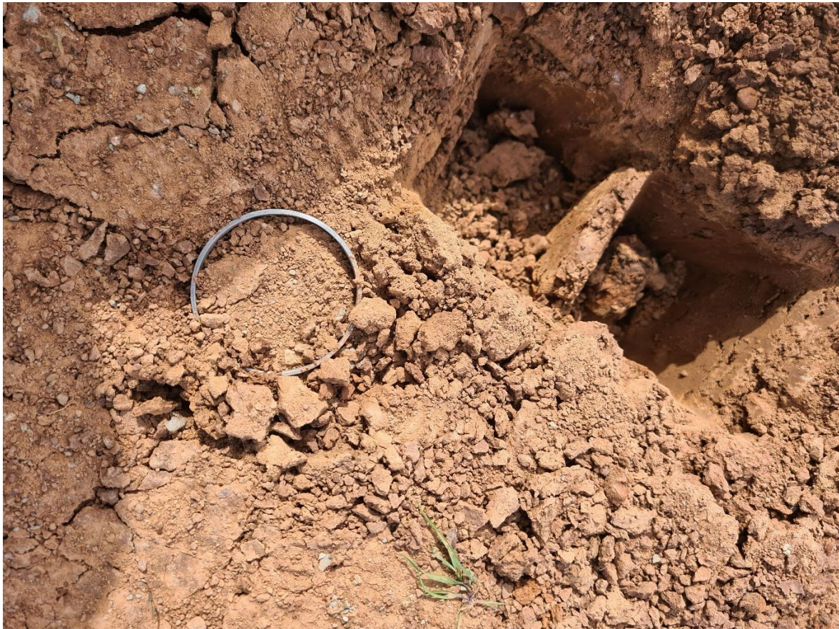
Figure 8: Cylinder located in soil prior to collection and sending off to the Laboratory for testing
