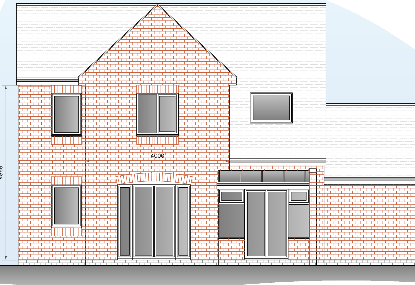
PROPOSED REAR ELEVATION (SCALE 1:50)
