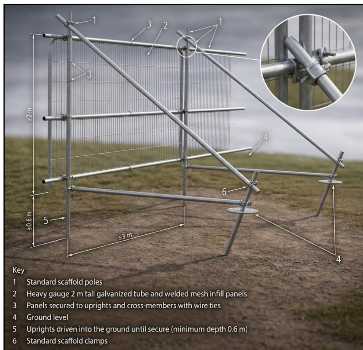
Figure 2: Default specification for protective barrier
