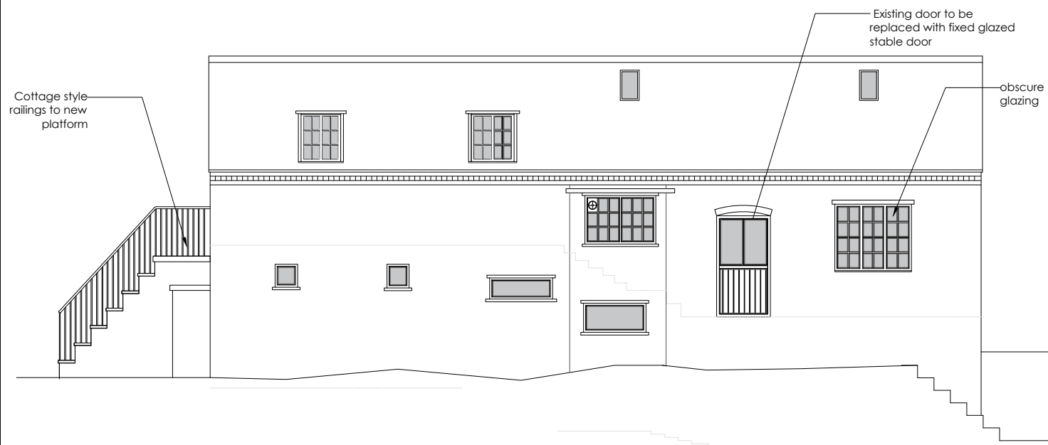
Proposed : South East Elevation scale 1:100
