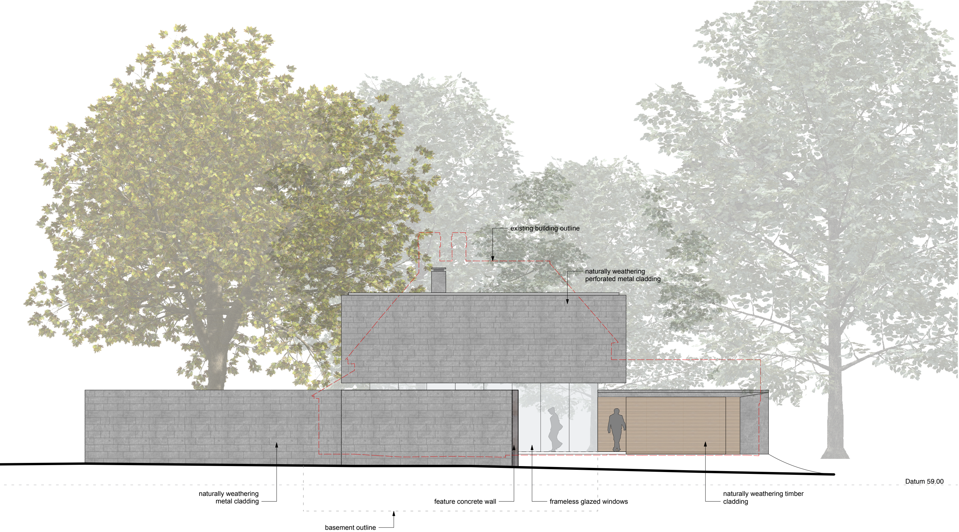
proposed north east elevation scale 1:100@A3
