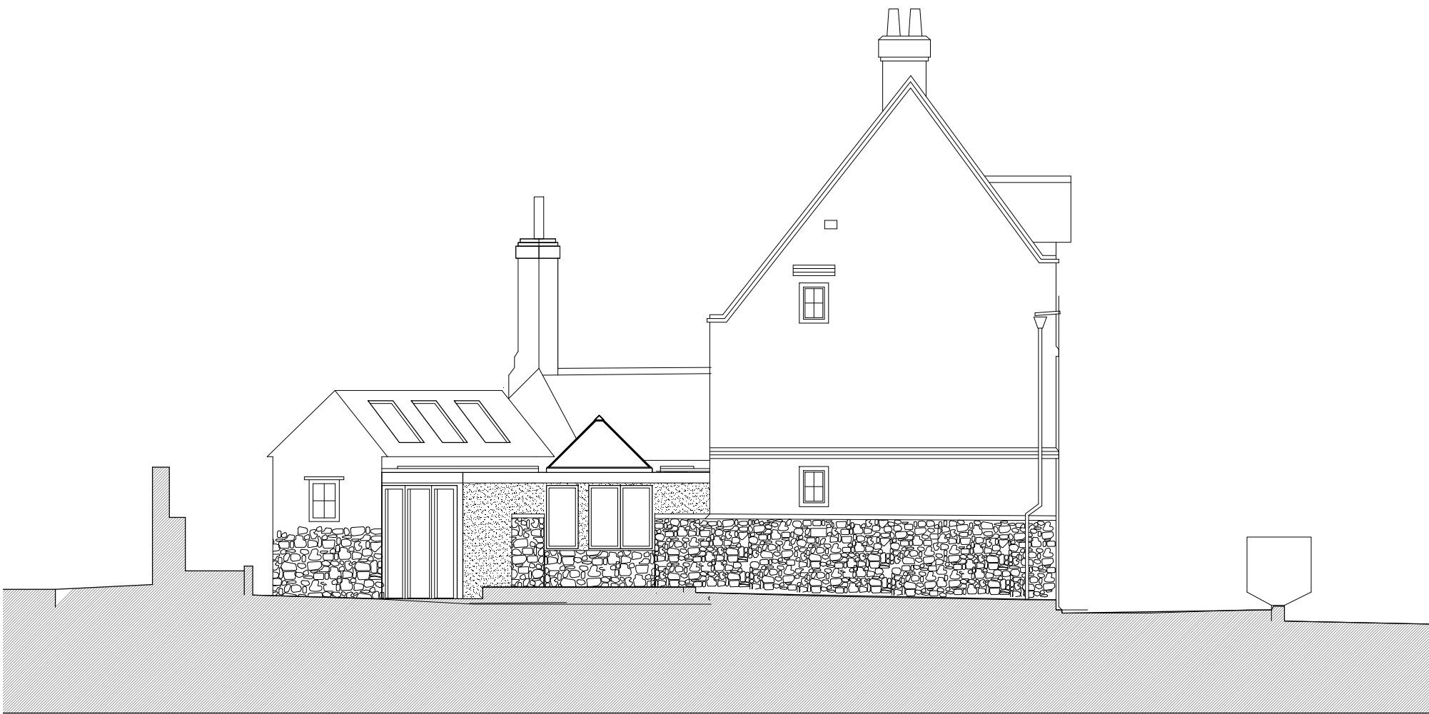
SIDE ELEVATION SHOWING EXISTING STONE WALL
