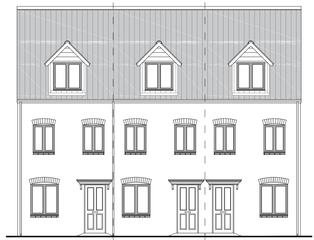
Front Elevation (Terrace)
