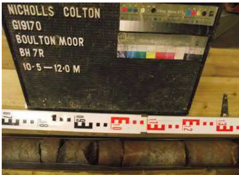
Core Run 3 – 10.50-12.00m (Siltstone & Mudstone).
