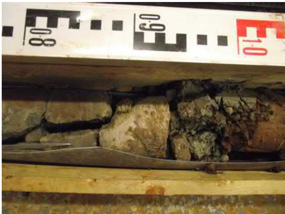
Core Run 3 - 13.00-14.50m (Sandstone & Clayey silt).
