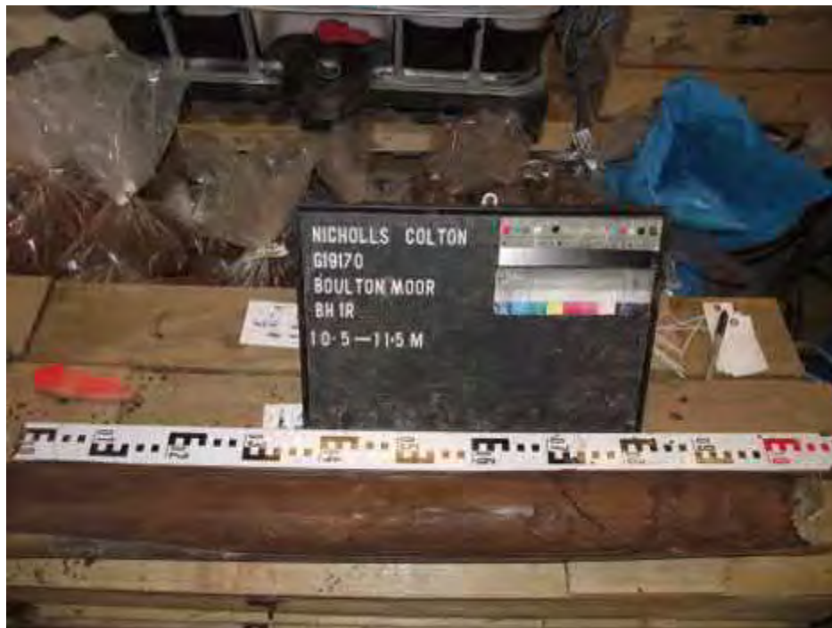
Windowless Sample Liner 10.50-11.50m.
