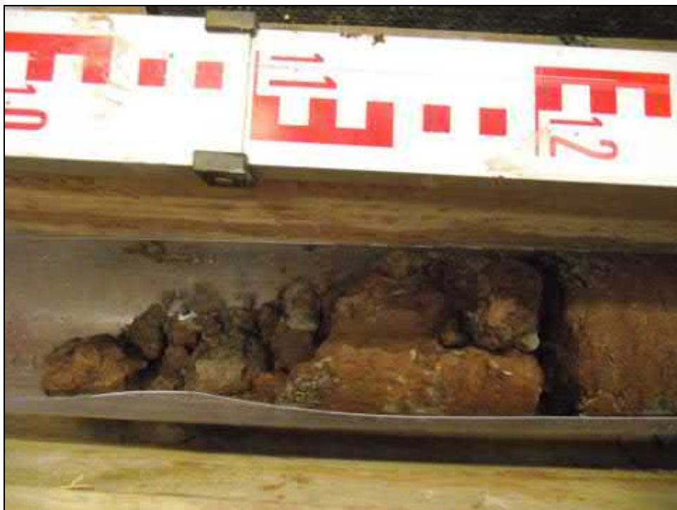
Core Run 3 – 13.50 – 15.00m (Silty clay).
