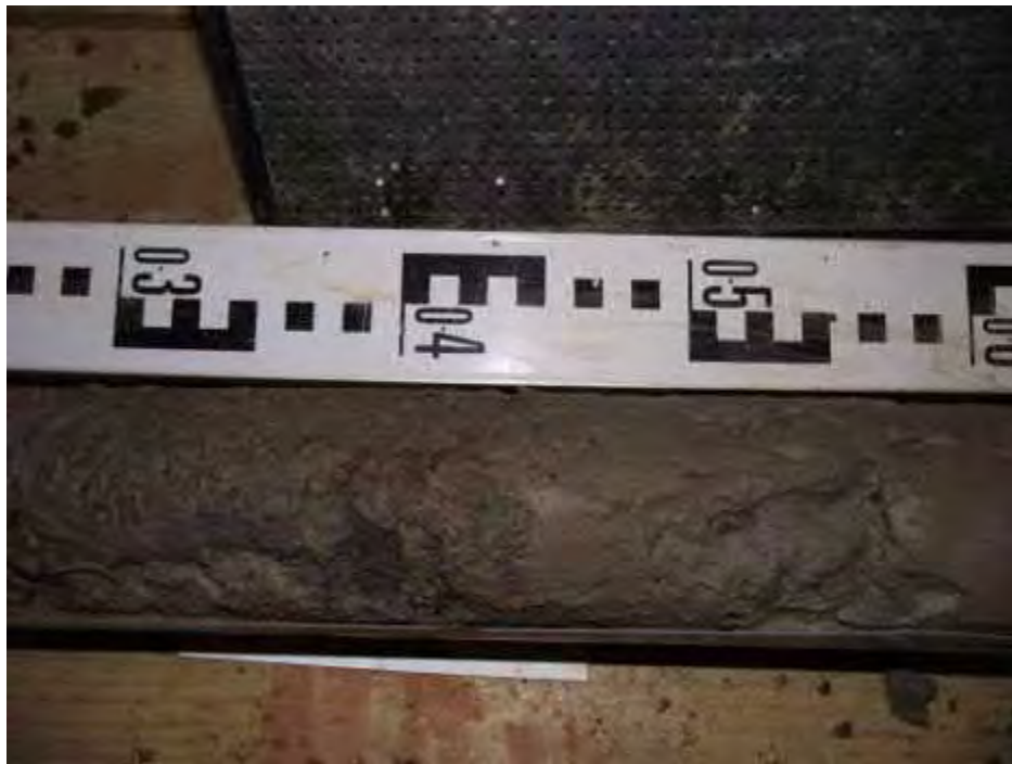
Windowless Sample Liner 9.00-10.00m (Silty sand & Sandy silt).
