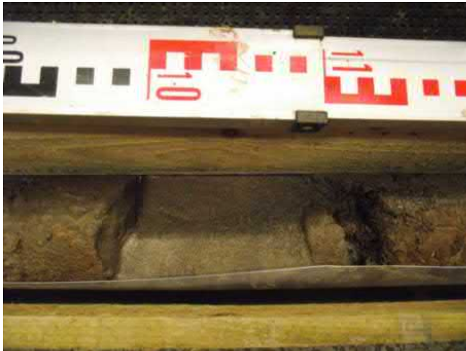
Core Run 2 - 12.00 - 13.50m (Sandy clayey silt, sand & siltstone).
