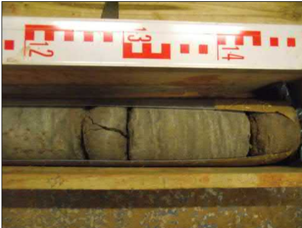
Core Run 4 – 14.50 – 16.00m (Sandstone).
