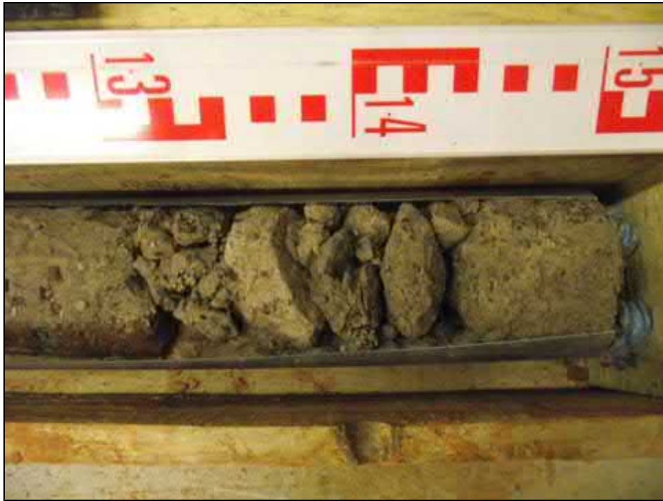
Core Run 2 – 7.50-9.00m (Sandstone).
