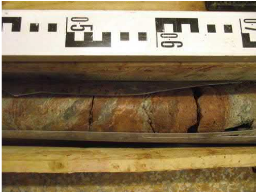
Core Run 3 - 13.00-14.50m (Sandy siltstone & Sandstone).
