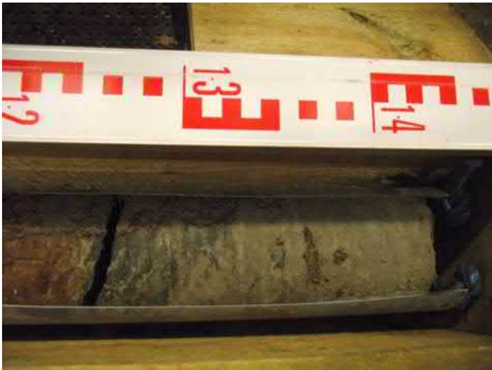
Core Run 2 - 12.00 - 13.50m (Sandy siltstone & Sandstone).
