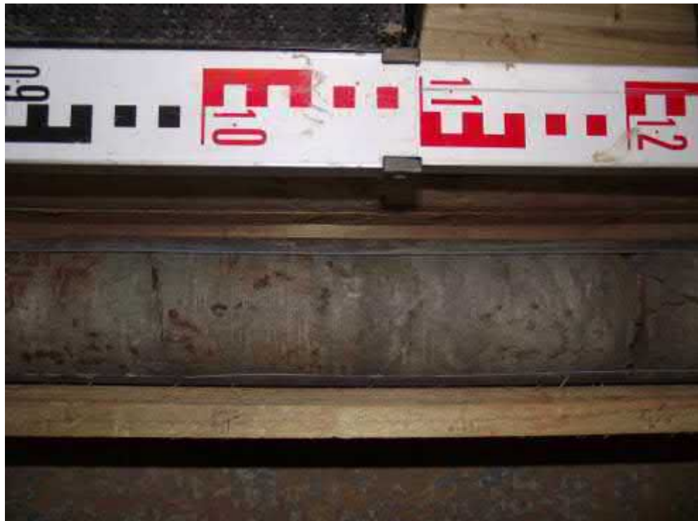
Core Run 4 – 14.50 – 16.00m (Sandstone).
