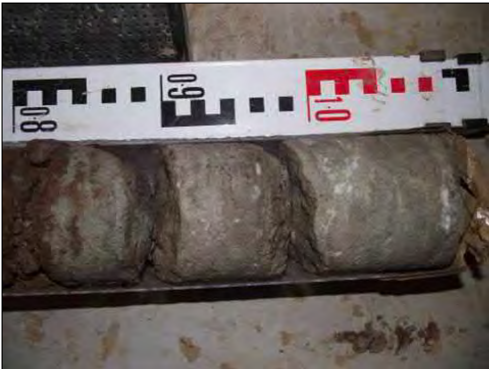
Core Run 4 - 9.00-10.00m (Sandstone).
