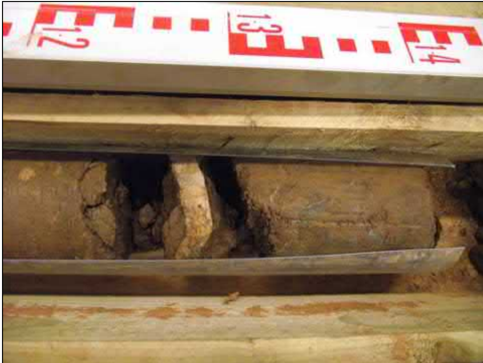
Core Run 4 - 12.00 - 13.50m (Mudstone including Gypsum band.
