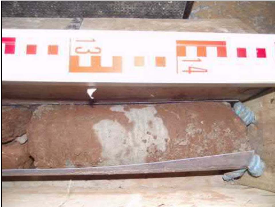
Core Run 3 – 13.50 – 15.00m (Sandstone).
