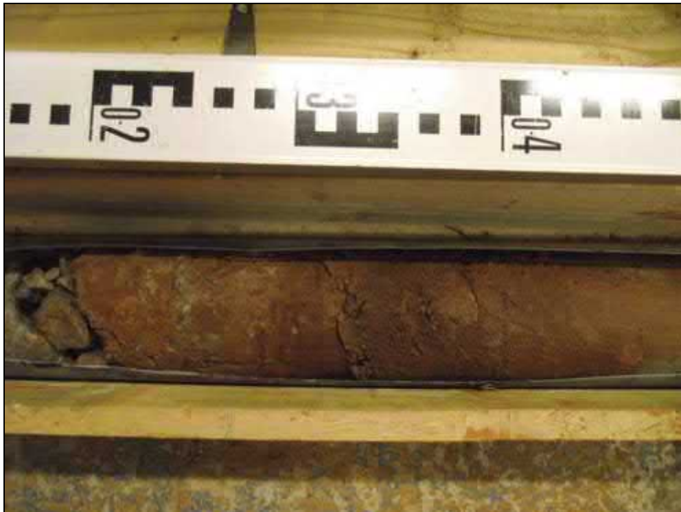
Core Run 4 – 14.50 – 16.00m (Sandy clayey silt & sandy Siltstone).
