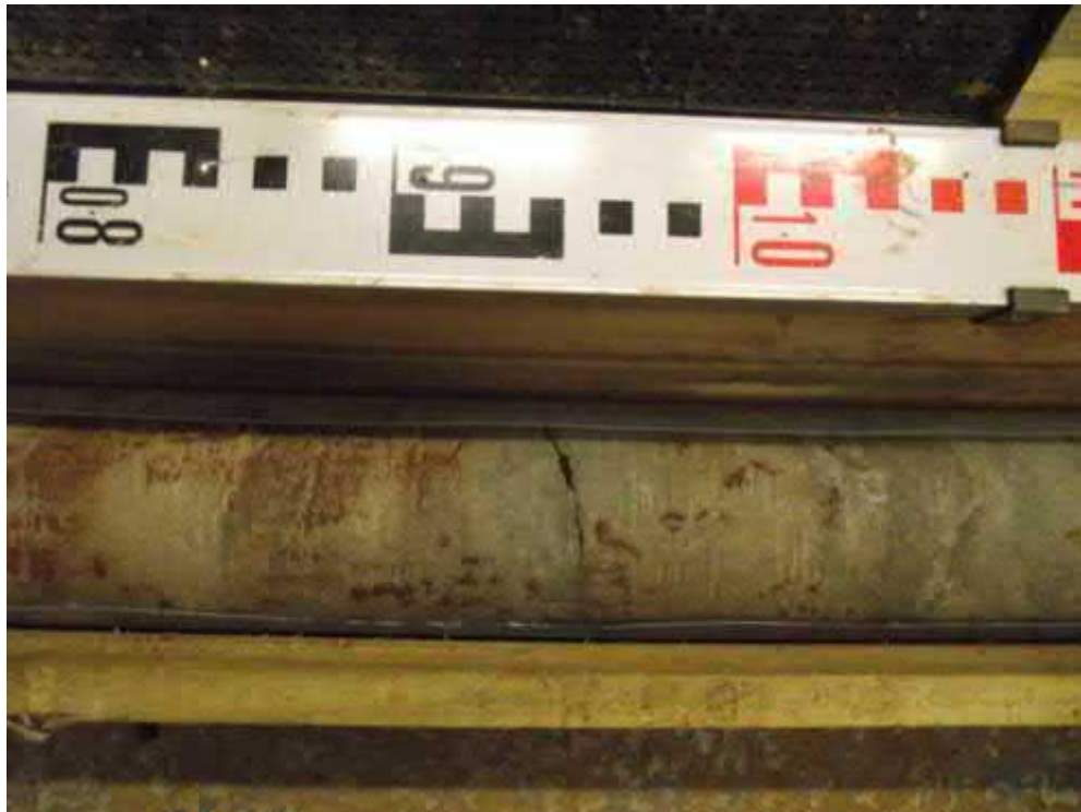
Core Run 4 – 14.50 – 16.00m (Sandstone).
