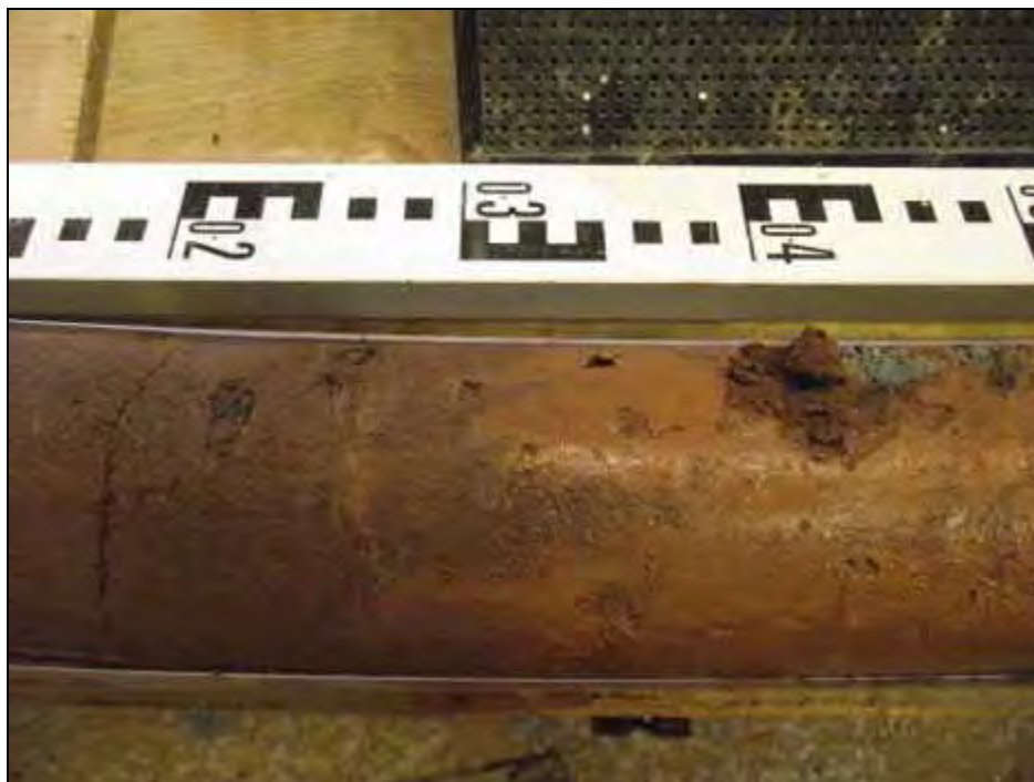
Windowless Sample Liner 9.00-10.00m (Sand & Sandy silt).
