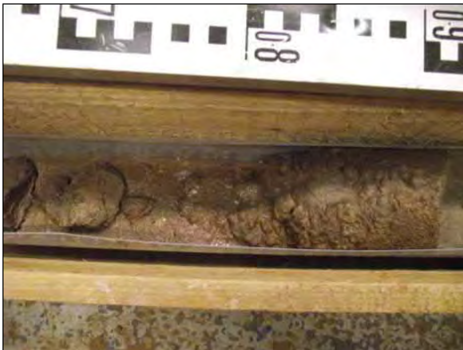
Core Run 2 - 12.00 - 13.50m (siltstone, sand & clayey silt).
