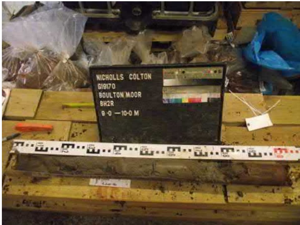
Windowless Sample Liner 9.00-10.00m.
