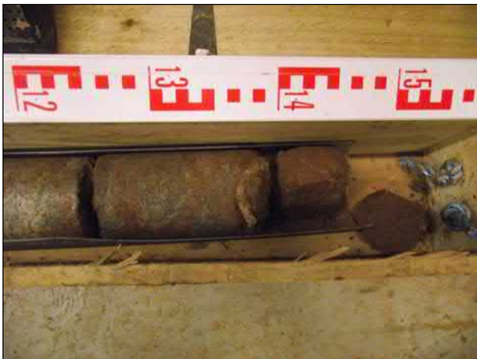
Core Run 3 – 10.50-12.00m (Mudstone including Gypsum vein).
