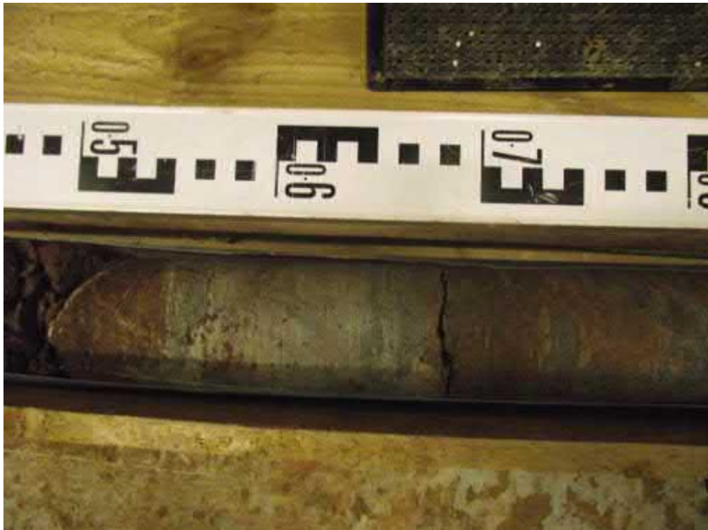
Core Run 5 – 13.50 – 15.00 (Mudstone with Gypsum vein) .
