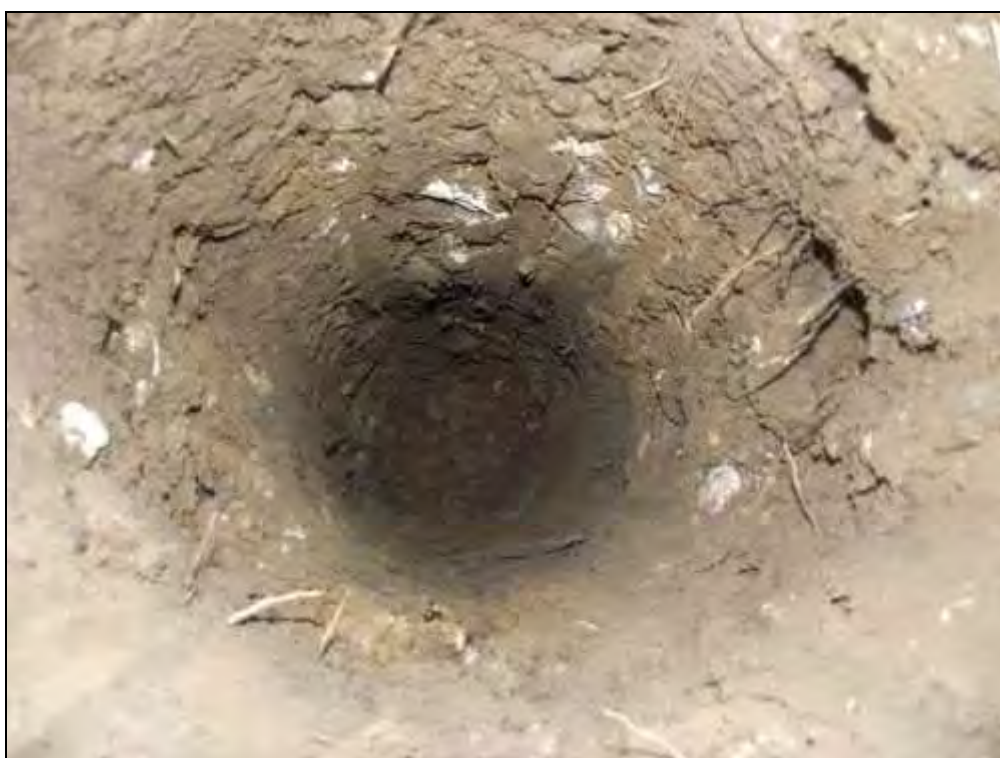
Borehole BH3: Starter Pit Internal View.
