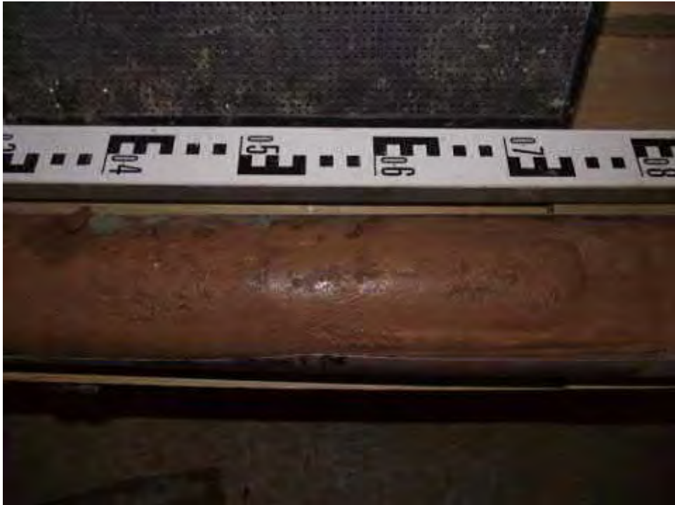
Windowless Sample Liner 9.00-10.00m (Sandy silt).
