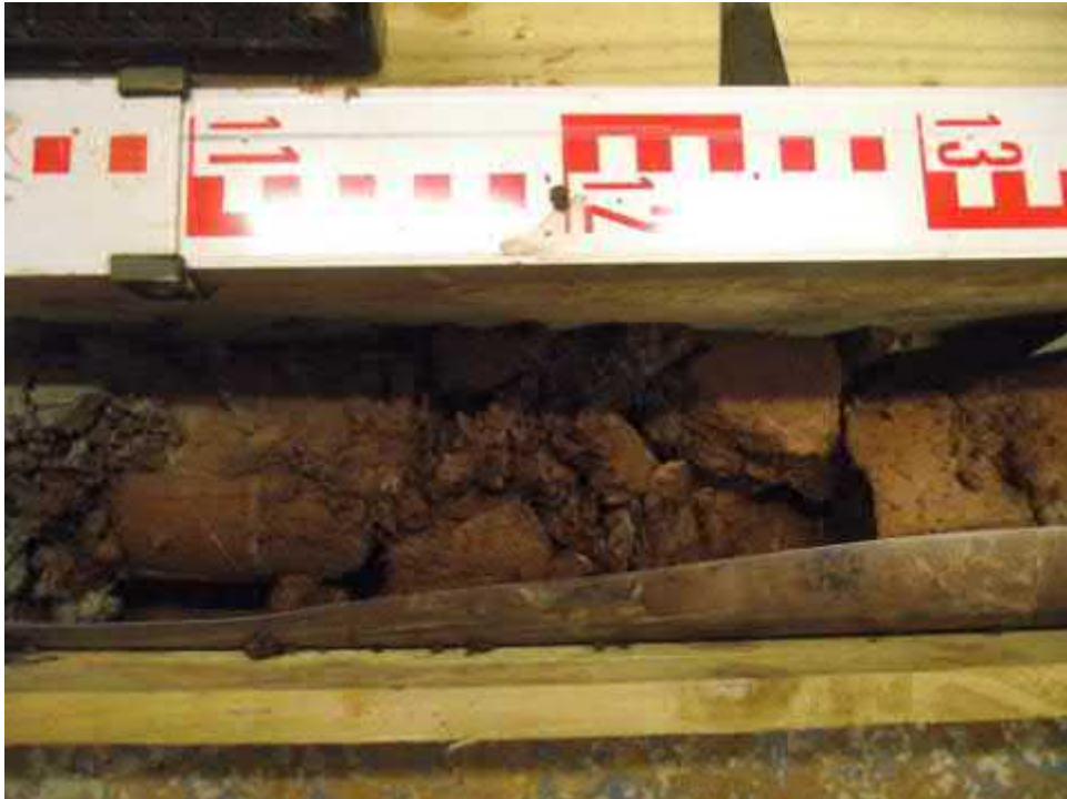
Core Run 3 - 13.00-14.50m (Clayey silt & Mudstone).
