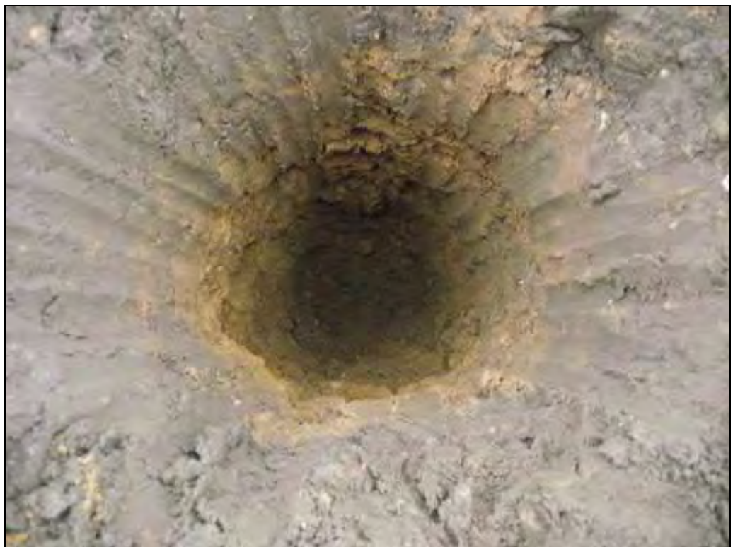
Borehole BH9: Starter Pit Internal View.
