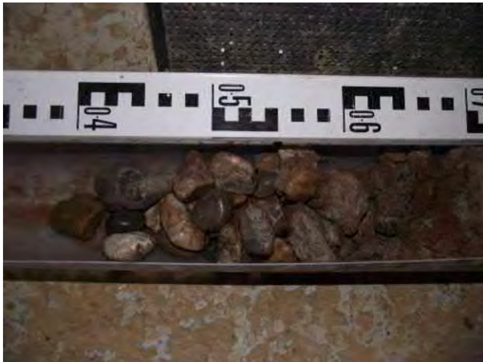
Core Run 4 - 9.00-10.00m (Conglomerate – recovered as pebbles with sand having washed away).
