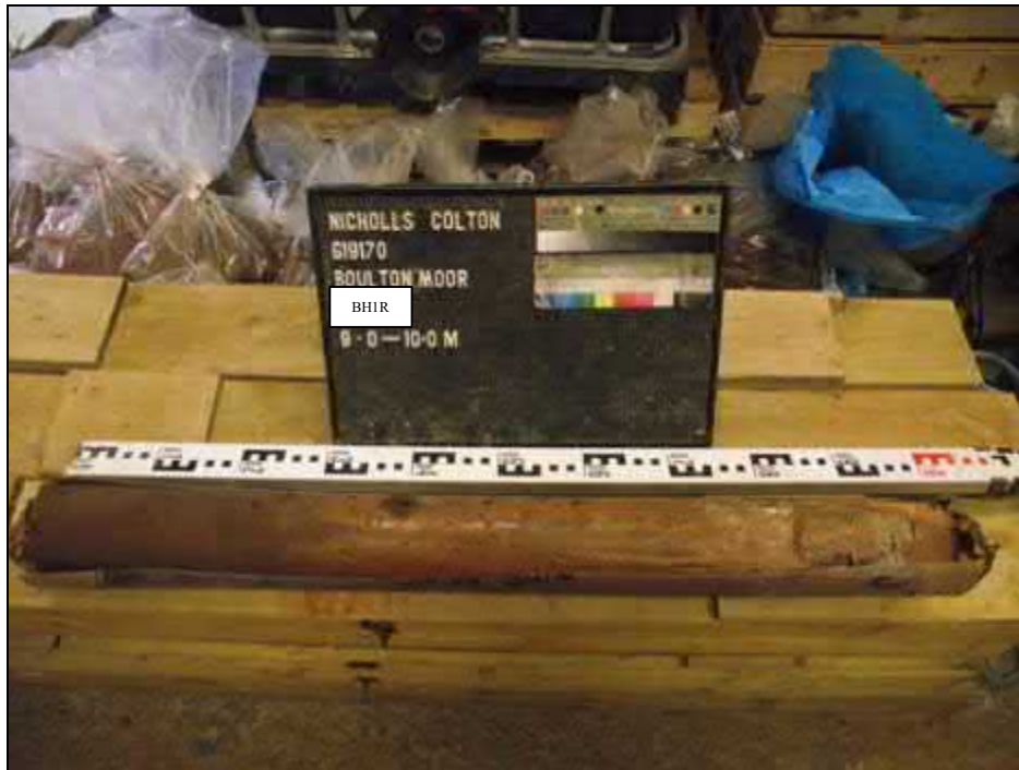
Windowless Sample Liner 9.00-10.00m.
