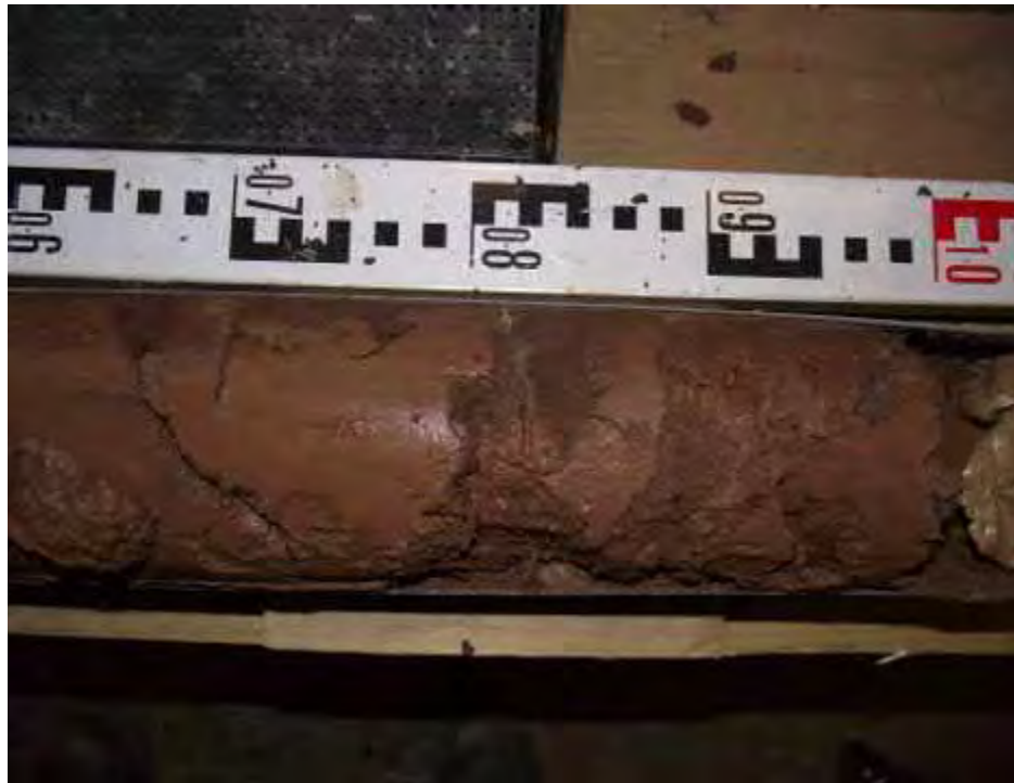
Windowless Sample Liner 10.50-11.50m (Clayey Silty sand).
