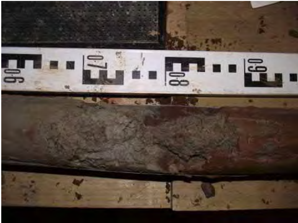
Windowless Sample Liner 9.00-10.00m (Silty sand & Sandy silt). Note: Windowless Sample Liner 10.50m-11.50m (Liner shredded soil placed into sample bag).
