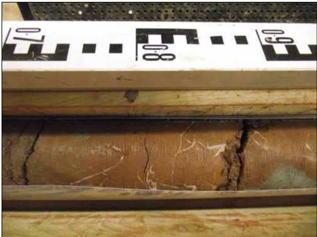
Core Run 4 - 12.00 - 13.50m (Mudstone including Gypsum veins).
