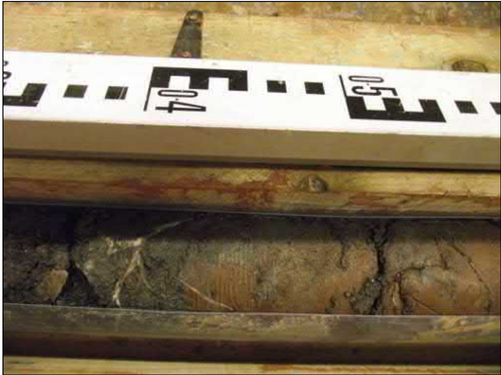
Core Run 4 - 12.00 - 13.50m (Mudstone including Gypsum veins).
