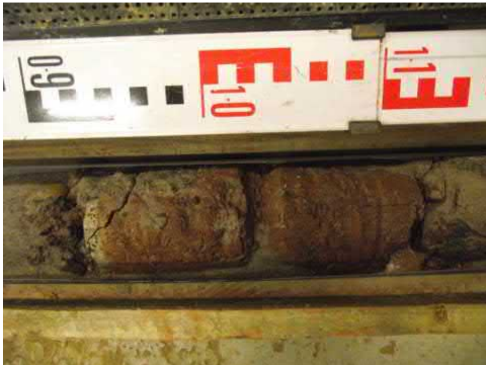
Core Run 2 – 7.50-9.00m (Clayey silt).
