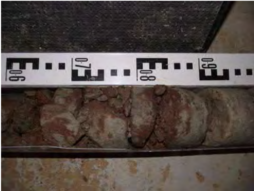
Core Run 4 - 9.00-10.00m (Sandstone).
