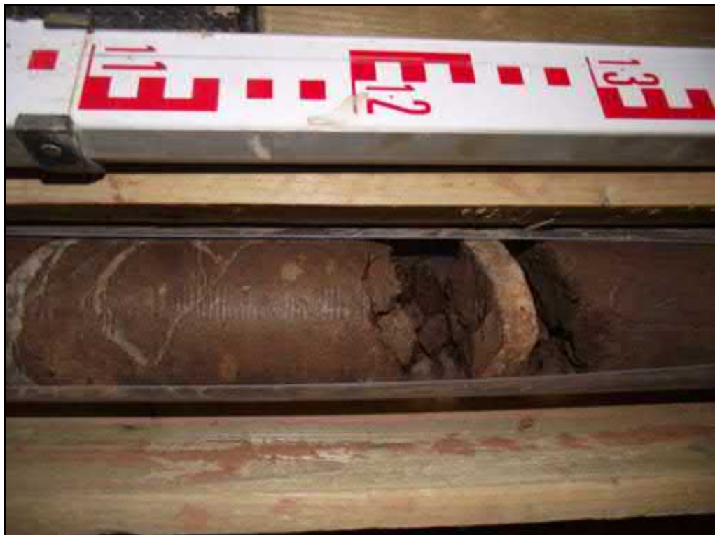
Core Run 4 - 12.00 - 13.50m (Mudstone including Gypsum band and veins).
