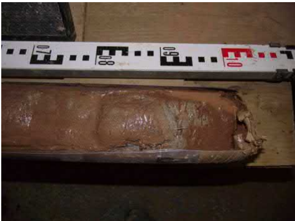
Windowless Sample Liner 9.00-10.00m (Sandy silt).
