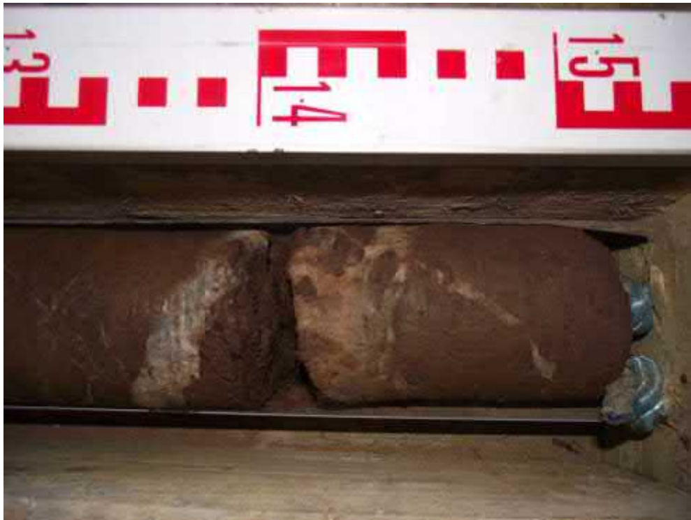
Core Run 5 – 13.50 – 15.00 (Mudstone & Gypsum bands/veins).
